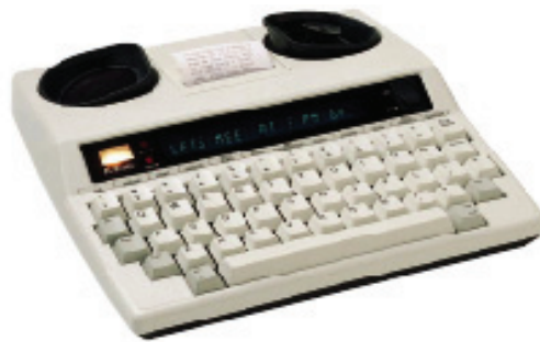
Figure 18. Ultratec Superprint 4425 TTY.
